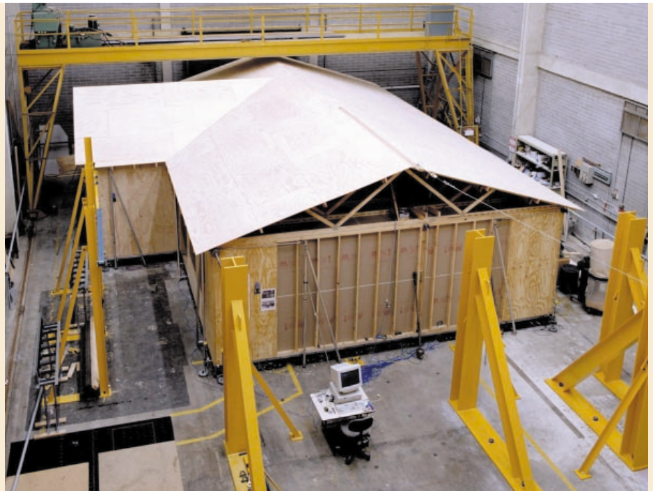
The research team at CSIRO Building Construction and Engineering built a house in their laboratory to gauge its response to loading scenarios caused by natural disasters. The results form the basis of a model that can be used to optimise the strength of buildings.
