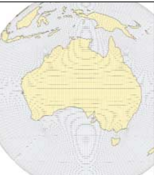
The ocean-atmosphere model simulates climatic processes at a horizontal grid spacing of two degrees and divides the atmosphere into nine layers.
