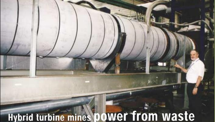
new hybrid turbine system that uses reject coal and methane gas to generate electricity could help 'green' the mining industry and reduce Australia's greenhouse gas emissions.
