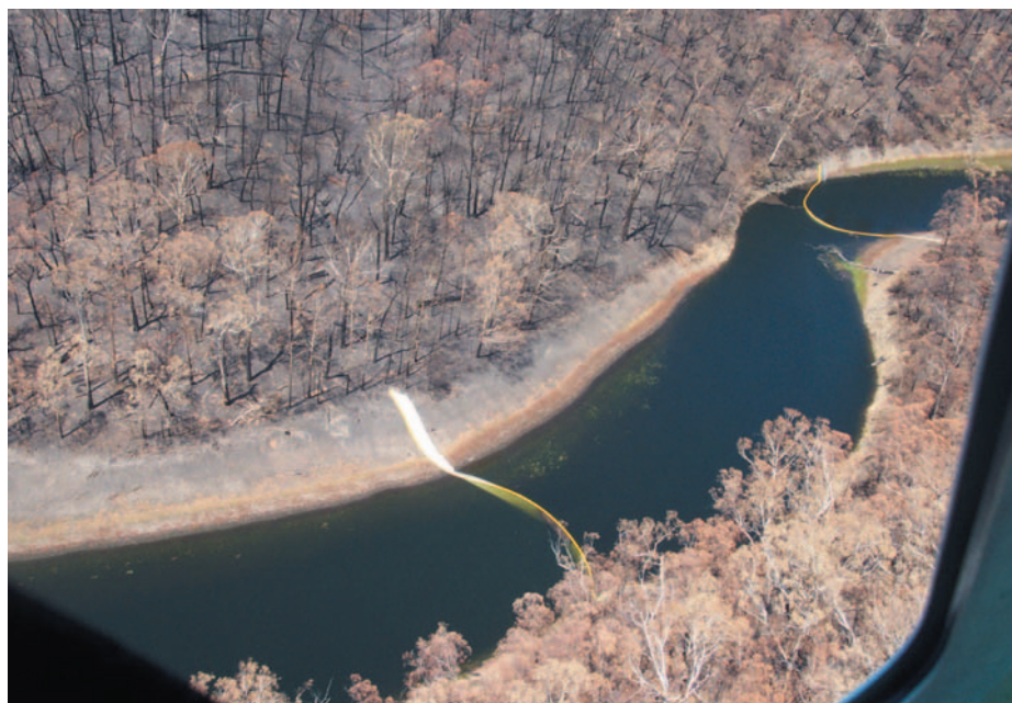
Double silt booms at the top end of Bendora Reservoir, part of Canberra's once-pristine water supply catchment.
