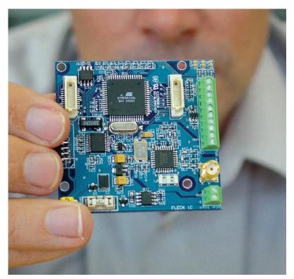
Potential applications in environmental monitoring, including waterways and oceans: The CSIRO-developed FLECK module is a low-cost embedded sensing and computing device with ad hoc wireless capability. It consists of a low-power central processing unit with additional off-chip flash memory and a radio receiver. Each FLECK has circuitry to charge a battery from a solar cell, and sensors for battery, solar and temperature levels built directly into the base platform as standard.
