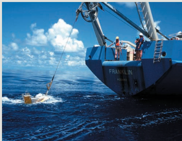
CSIRO's integral marine research vessel the RV Franklin deploys a SeaSoar ocean sampler. CSIRO Marine and Atmospheric Research
