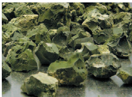
Solid algal cake, formed after GreenFuel's dewatering process, can be used to produce a range of valuable end products, including fuels, from the oils, proteins and carbohydrates in the algae. GreenFuel Technologies Corporation
