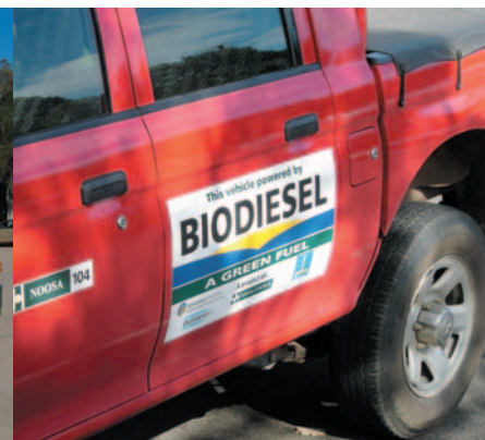
Noosa Council vehicles took part in a biodiesel trial that showed that the use of B20 biodiesel in the Council's work and waste collection vehicle fleet is likely to lead to significant reductions in particulates and CO 2 emissions. Noosa Shire Council
