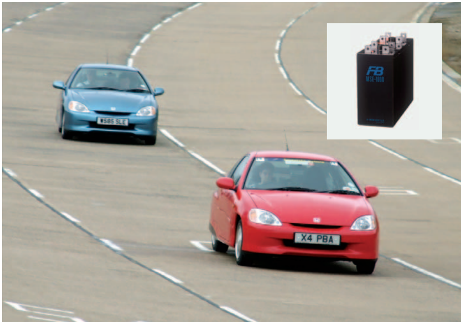
The UltraBattery (inset) may not only power hybrid electric cars – such as the red Honda shown here, driven for more than 145 000 km in a UK trial – but also smooth out short-term variations in wind energy. Advanced Lead-Acid Battery Consortium
