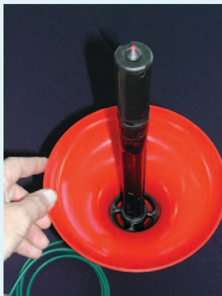
The FullStop wetting front detector knows when soil is wet enough and shuts off irrigation. CRC Irrigation Futures/Measurement Engineering Australia
