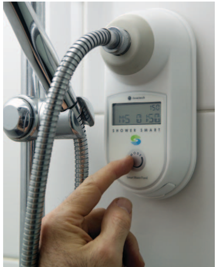
A smart shower meter being developed by Invetech and Victoria's Smart Water Fund: the OECD review of Australia's environmental performance suggested higher water pricing in urban areas to encourage more efficient use. Invetech Pty Ltd
