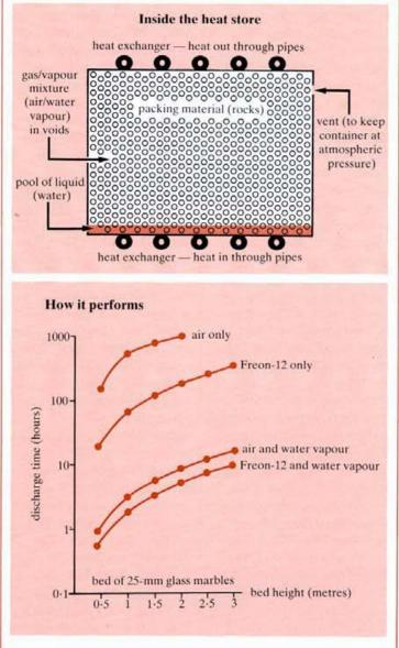
The graph shows estimated times to discharge 80% of the store's energy (a measure of its heat conductivity) for various gases and vapours. Use of a condensing vapour (water vapour) increases heat conduction considerably. The experimental heat store: a tank filled with glass marbles, some water, and air. It's heated by electricity at the bottom, and crisscrossed by temperature sensors.
