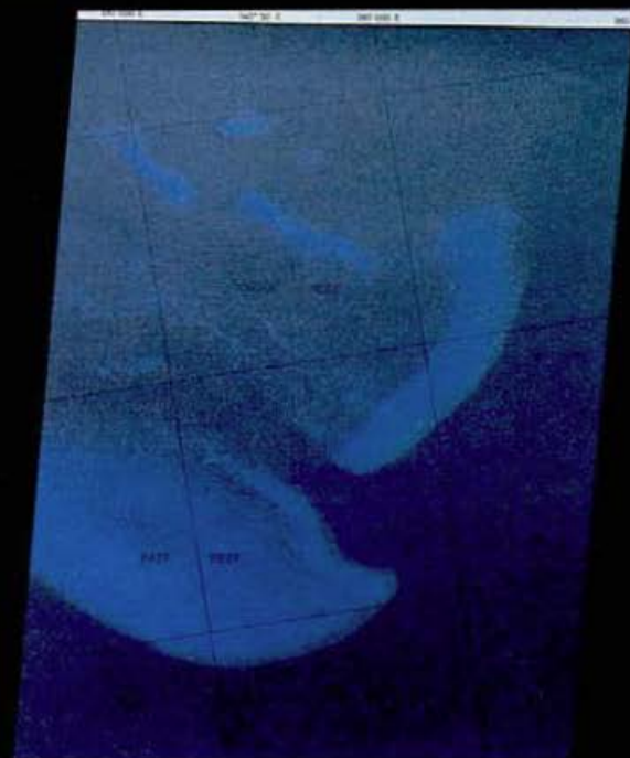
Tongue and Batt Reefs, near Cairns, as seen by Landsat. The image has been rectified: geometric distortions have been eliminated and map co-ordinates drawn in.
