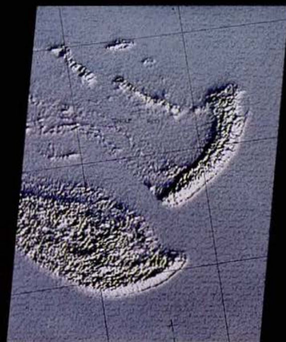
Getting the computer to shadow the Reefs as if illuminated from the south-east gives this 'exposure image'. It provides a texture that indicates the Reefs' exposure to the south-east, from which prevailing winds come.
