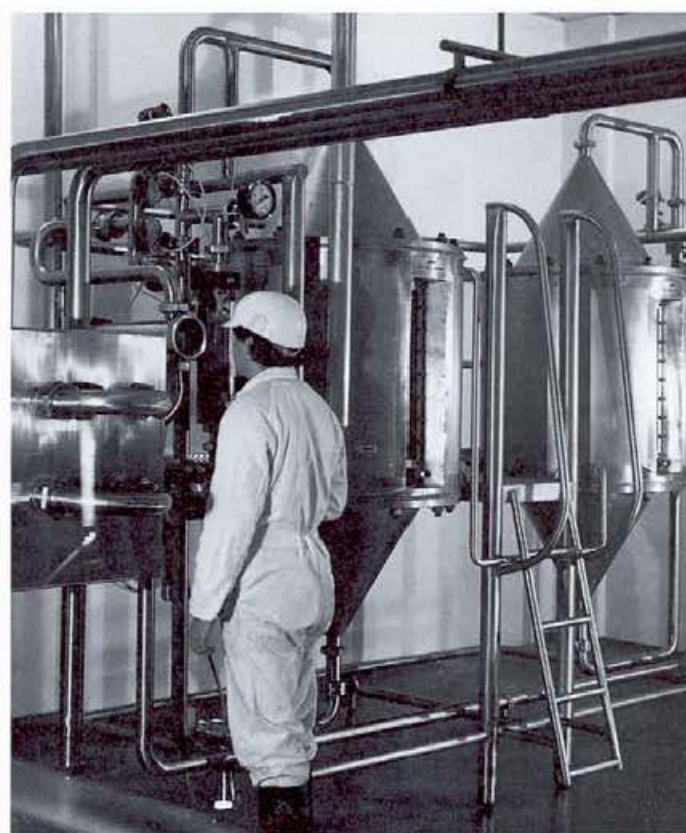
The Drouin factory's equipment for splitting lactose.
