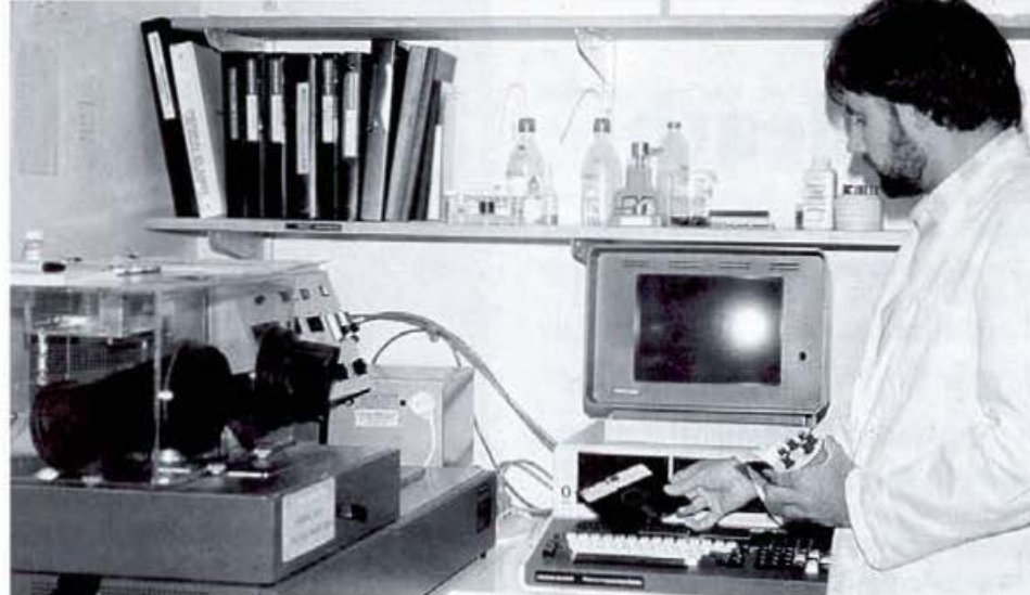
Dr Ted McMurchie operating the differential scanning calorimeter that enabled him to measure precisely the phase transition points of a variety of lung surfactants and lipid mixtures.
