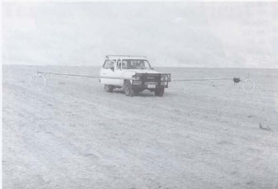
With transmitter and receiver loops mounted on a vehicle, conductivity readings covering 4 km can be made in an hour.
