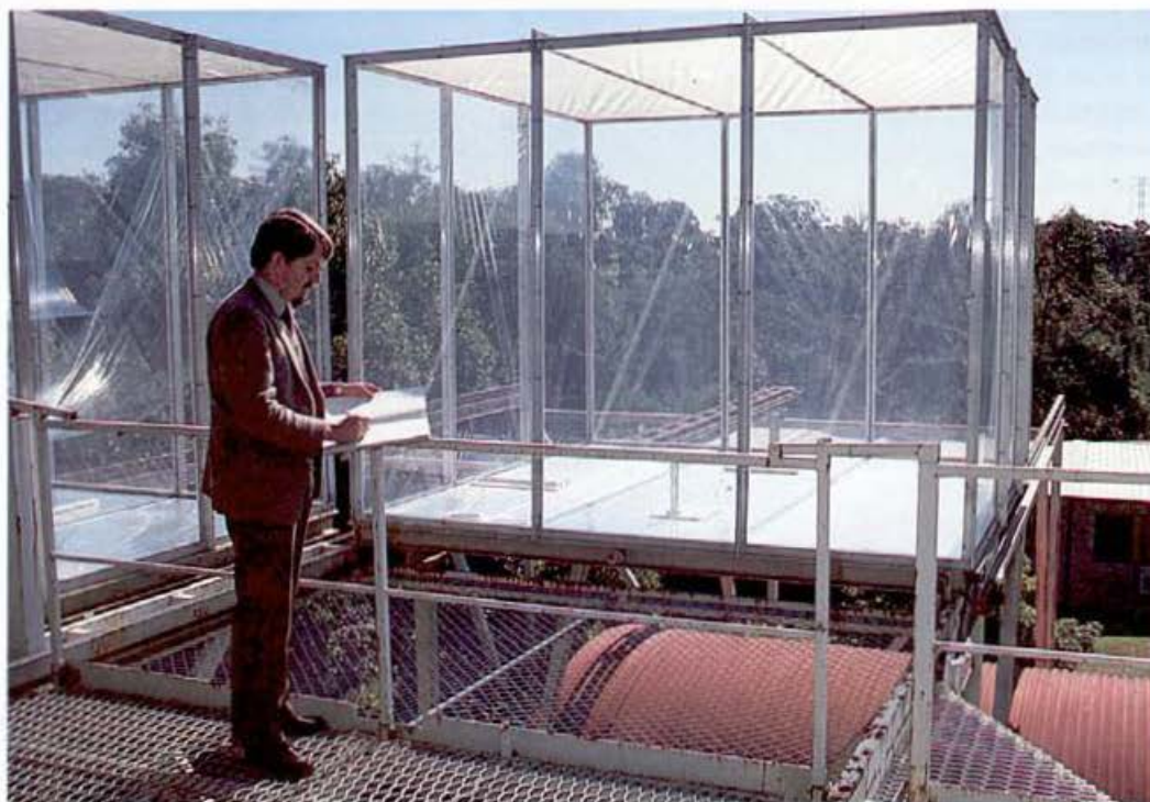
The CSIRO smog chambers (two transparent boxes that can be moved between full sun and full shade) provided the understanding of smog chemistry that allowed the new factory's effect on smog to be predicted.
