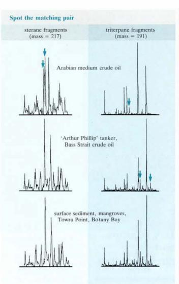
Yes, the molecular 'fingerprints' of the bottom pair in each column are virtually the same (the arrows show tell-tale differences from top traces). This indicates that oil from the offending spill came from Bass Strait, not the Middle East.
