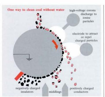
Mineral matter is conducting, while coal is not. So electric fields can separate one from the other, as illustrated. This electrodynamic method avoids using water and the problems that arise from trying to dry fine wet coal.
