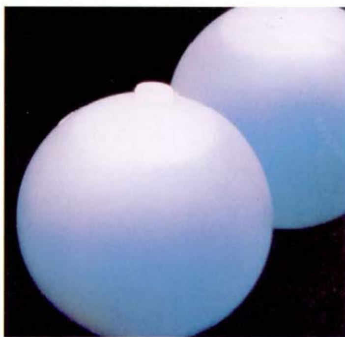
The polypropylene nodules, 77 mm in diameter, are filled with water or salt solutions of various types.
