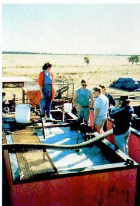
Scientists watch mixing of the nutrient solution that both feeds the bacteria down the well and determines what compounds they will release.
