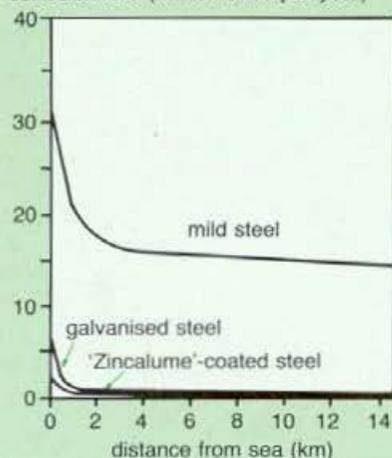
Mr King found a dramatic decrease in the rate of corrosion within the first kilometre from the sea. Because of this, he believes the Australian Standard Classification of a 'severe marine environment' should be limited to 2 km from the coast rather than the present 7 km.
