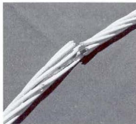
**Corroding electricity conductors are a major problem for electricity authorities. Mr King is working with the Electricity Trust of South Australia to find out in which parts of that State the transmission/distribution system is most susceptible.**
