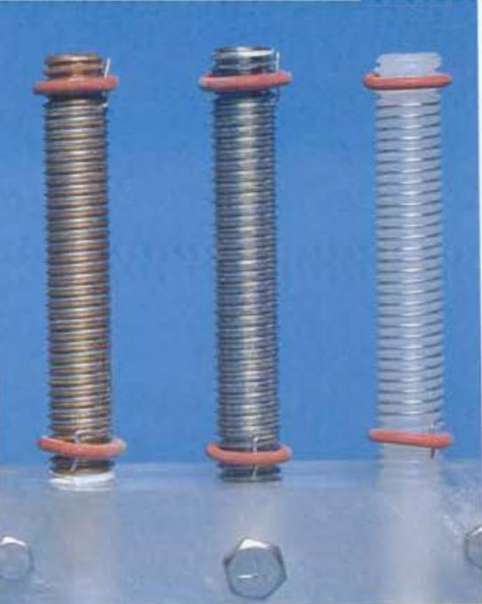
This 'wire-on-bolt' device (to be manufactured by CSIRO under the name 'ATCORR') provides a simple, quick means of assessing corrosion rates.
