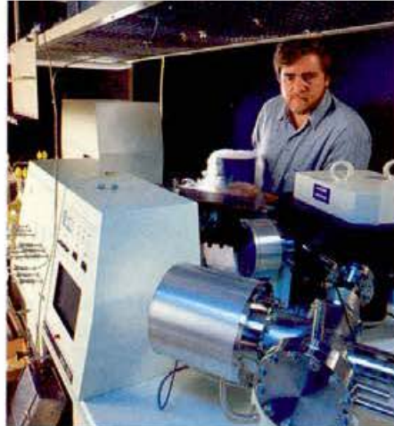
Dr Colin Allison with GASLAB's new high-precision mass spectrometer, used to study isotopes of greenhouse gases.
