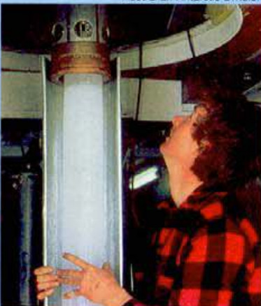
A glaciologist retrieves an ice core from a depth of 300 m in Law Dome, Antarctica. Air extracted from the ice at ICELAB is measured in GASLAB to study past changes in the composition of the atmosphere.
