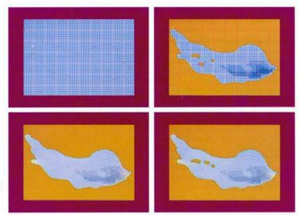
How NESSIE 'constructs' an artificial lake. First the designer draws the lake's physical parameters: its boundaries, shallows and depths, and islands. Then NESSIE plots the flow of water from one or more entry points, around or over obstacles, and shows residence times. A planner can assess how well a lake is 'working' by comparing flow patterns and residence times; he or she can even manipulate lake design to achieve optimum performance.
