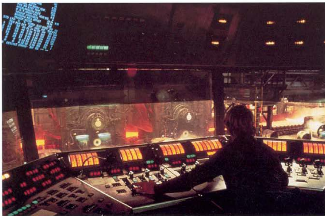
Inside BHP's hot strip mill. Rolling of steel slab into long sheets occurs here and at the cold-rolling mill, where mineral oil and tallow are used as lubricants. The mills roll about 1.5 million tonnes of steel a year.
