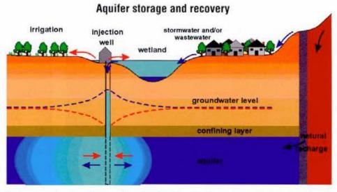
Stormwater and sewage effluent can be captured and treated at times of high flow, then stored deep underground in existing aquifers until needed. The main research challenge is to guard against contaminating the aquifers with chemicals and microorganisms.
