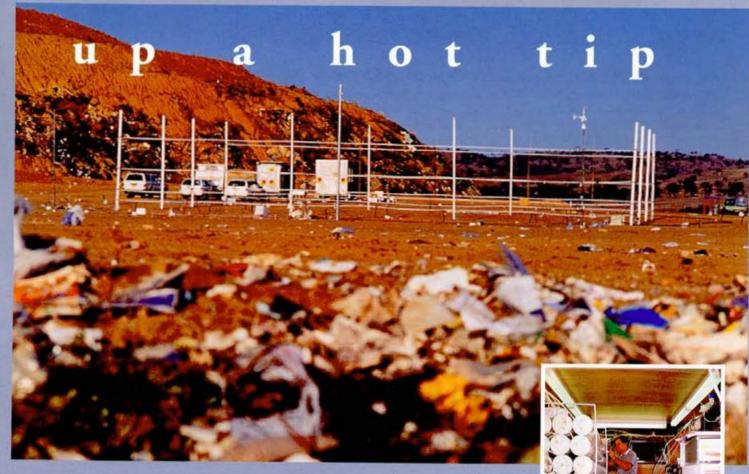
To calculate the amount of methane actually produced by the landfill, a trace gas budget was used. This involved subtracting the amount of methane carried into the trial area by the wind from the amount carried out. The difference is the amount of methane produced inside the 'fence'.
