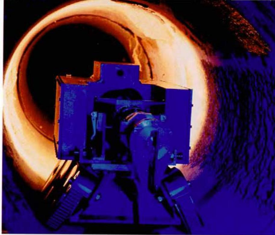
A small silver robot equipped with six wheels, laser and sonar scanners and an umbilical cord attached to an artificial brain has been inching its way through Melbourne's sewers. Disguised as Dr Who's faithful friend, K9, the device has inspected more than four kilometres of the city's underground pipes, assessing structural defects with unerring accuracy.
