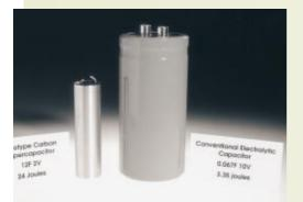
('Energy density' refers to the amount of energy the supercapacitor can store, which is small compared to batteries. 'Power density' refers to the amount of energy it can deliver in a specific time.)
