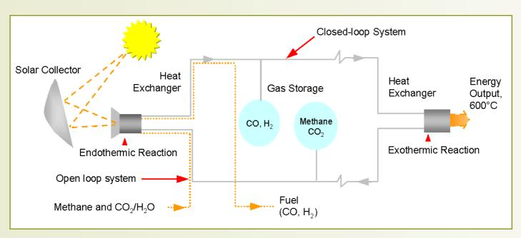
Carbon dioxide/methane reforming has a number of advantages over other thermo-chemical storage systems: it can be used in open and closed loop systems and it can utilise gas derived from natural gas, from coal-bed methane or from landfill.
